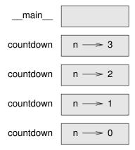
As usual, the top of the stack is the frame for \_\_main\_\_. It is empty because we did not create any variables in \_\_main\_\_ or pass any arguments to it.
