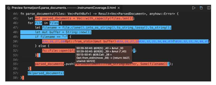
The image above shows one such example. The orange and blue backgrounds highlight alternating CoverageSpan s from the refined set. Hovering over a line expands the output on that line to show the MIR BasicBlock IDs covered by each CoverageSpan. While hovering, the CoverageSpan under the pointer also has a *tooltip* block of text, showing
