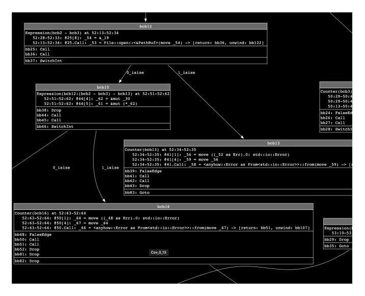
This image shows each BasicCoverageBlock as a rectangular *node*, with directional edges (the arrows) leading from each node to its successors(). The nodes contain information in sections:
